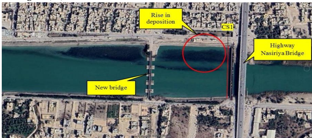
Figure (16): Shows the location of cross-section No. (1) and the effect of bridges on sedimentation conditions
