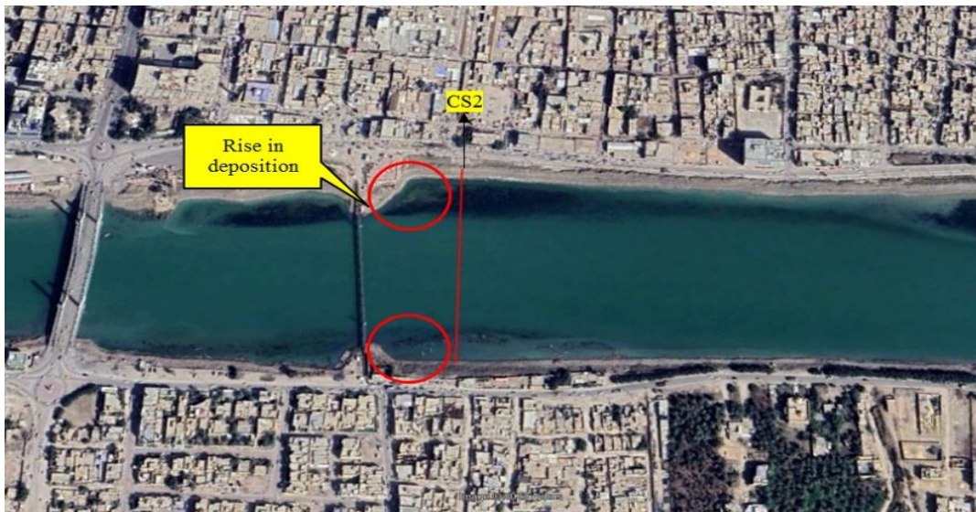
Figure (17): Shows the location of cross-section No. (2) and the effect of bridges on sedimentation conditions
